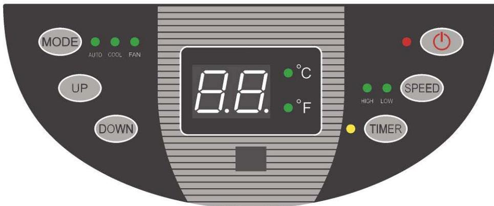
1. POWER button: press this button to turn on/off the unit.
